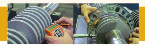
Testing and Alignment Services of V94.2, GE-F9 and MHI Turbine Fuel Injectors
